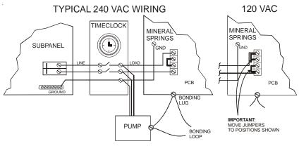
Note: Wire the pump directly to the timeclock--do not use the Mineral Springs as a junction box.
